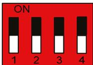
With the Dip Switches set in this configuration the unit is set to Multi Ramp mode (Two channel with five ramp up events and five ramp down events on channel A five ramp up events and five ramp down Events on channel B).
