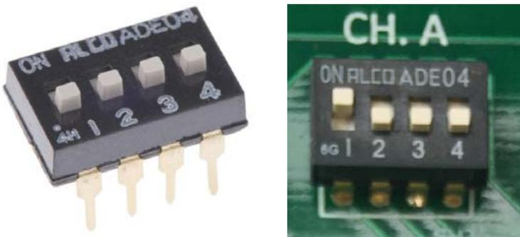
If **one** ALIS Dimmer is connected, then Dip SW 1 is set to ON.
